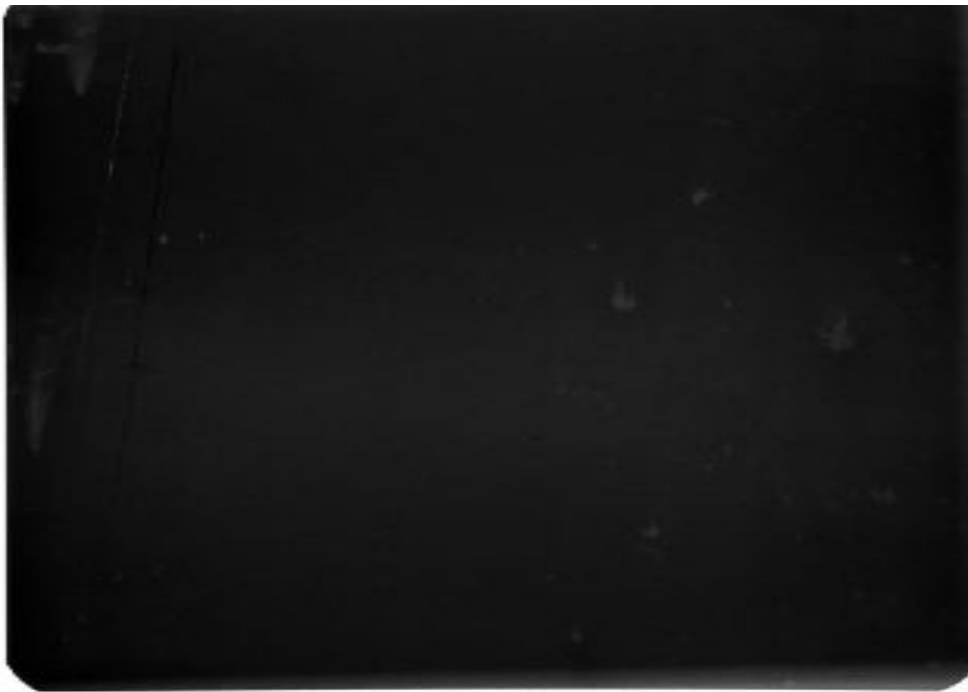
Radiography Film Exposed to x-ray at 48 kVp for 3.33s
