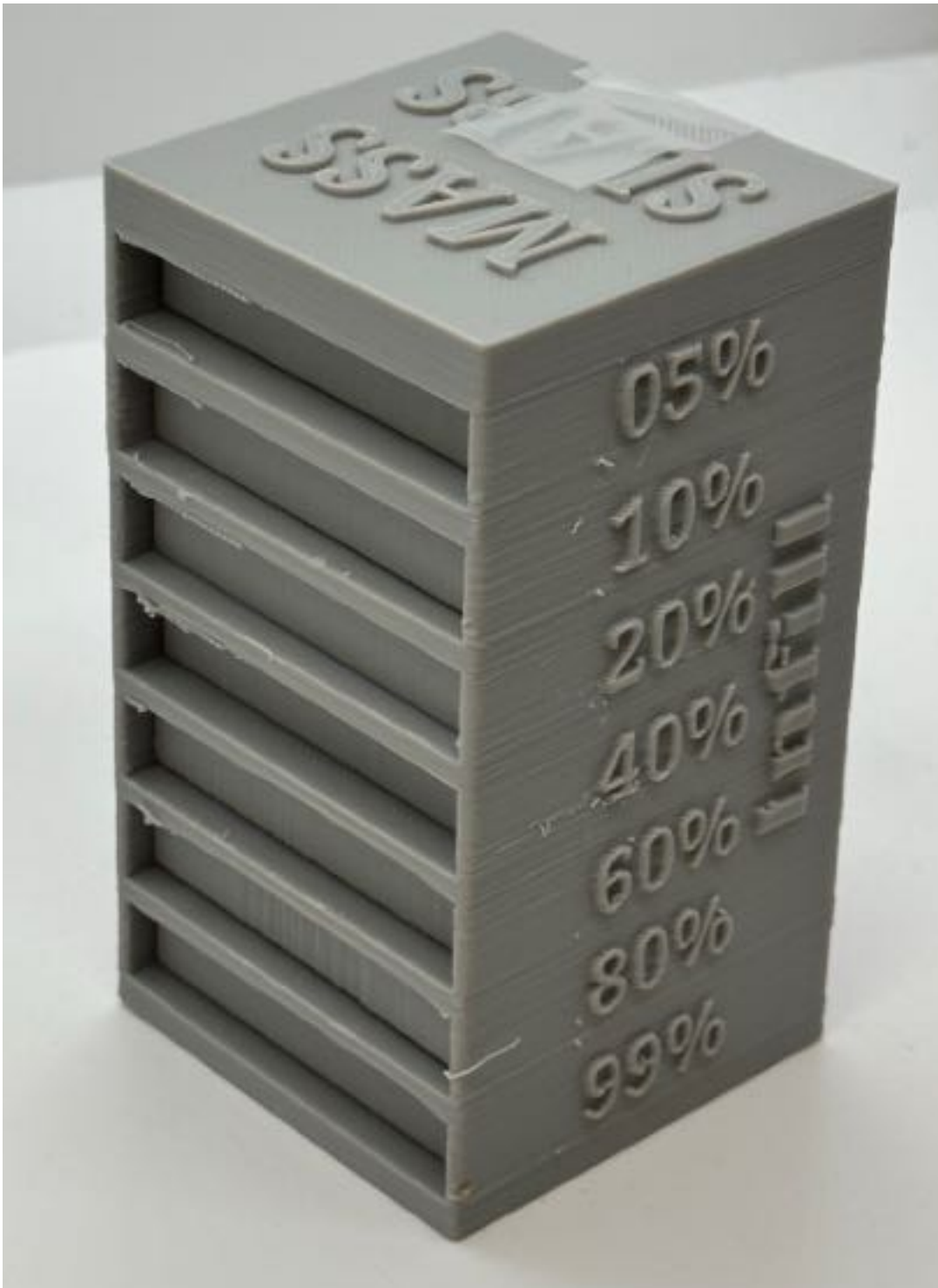
3D-Printed Blocks made of Gray PLA with Different Infill Percentages
