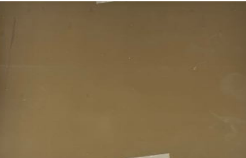
Film Exposed to x-ray at 48 kVp for 3.33s
