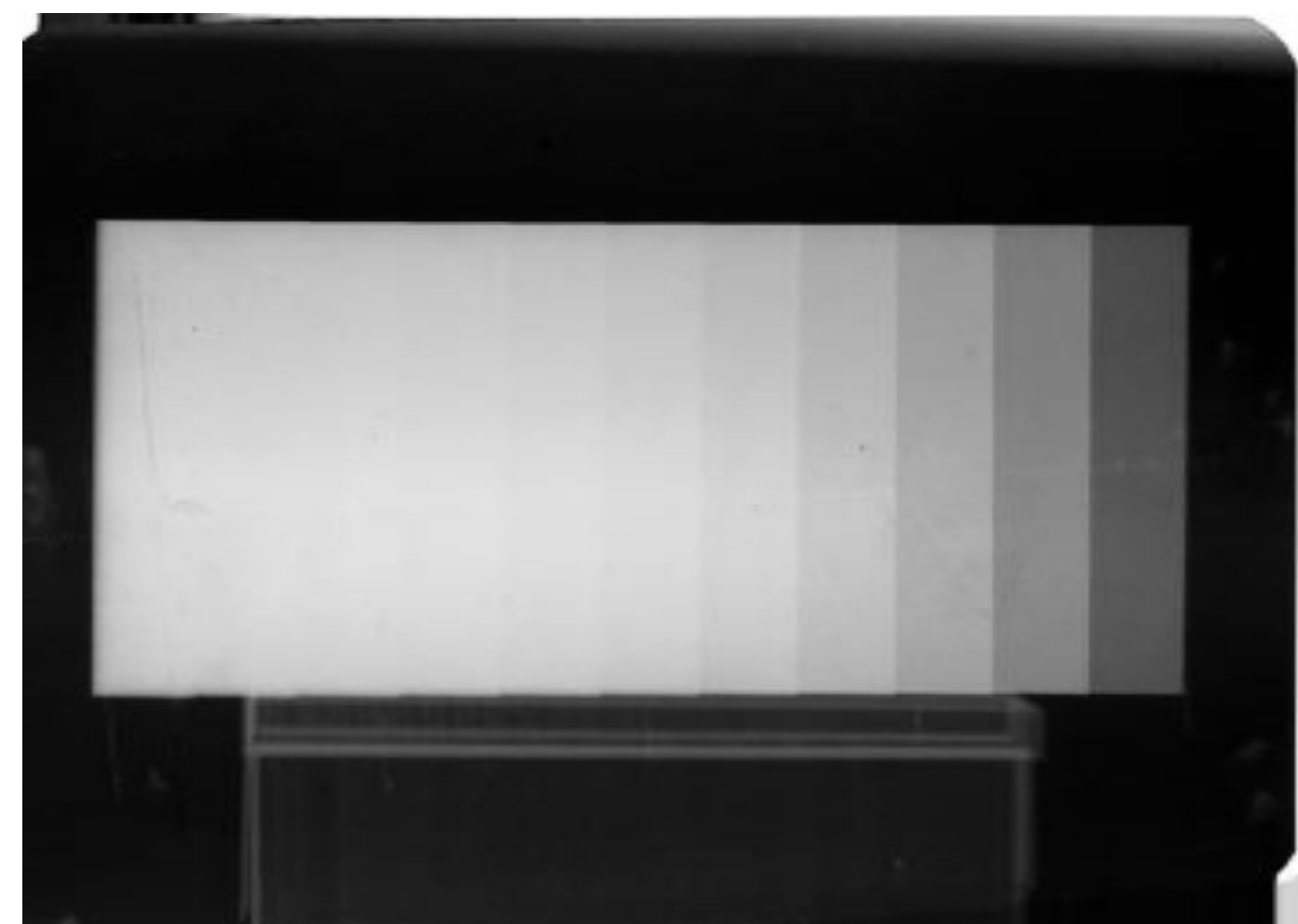
Scanned Radiography of the Al Step-Wedge
